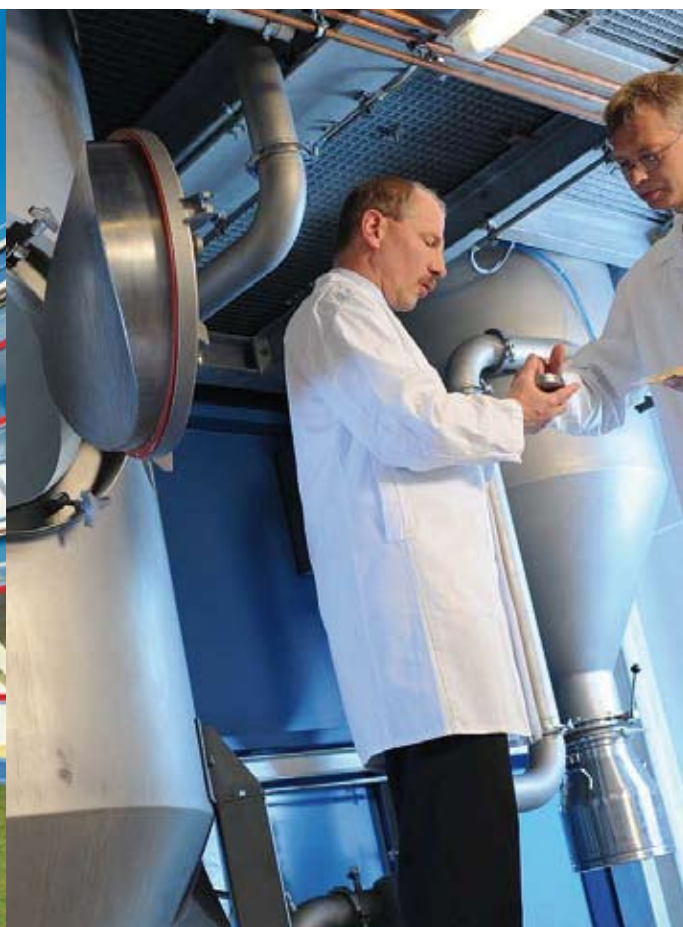
Product development with the pilot spray tower
